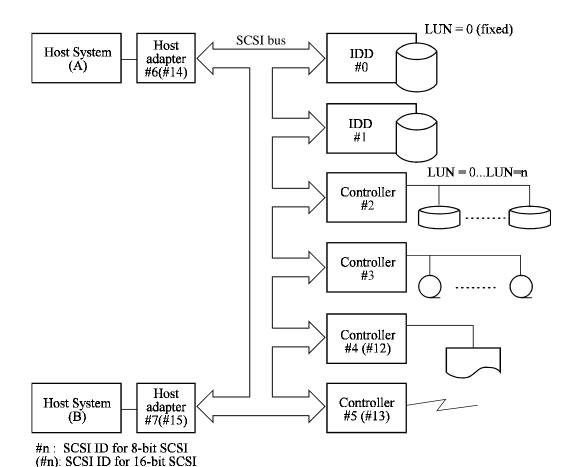
Figure 1.4 System configuration
